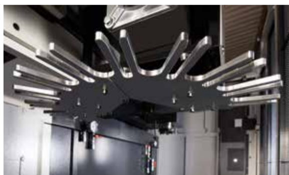
Electrode changer of the EA8S model with ten magazine pockets
