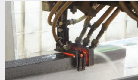
Induction hardened solid box guideways with linear scale feedback on all axes with twin ballscrew design in X & Y axes.
