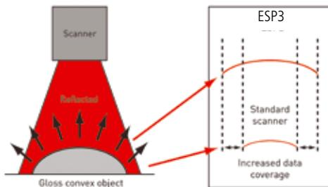
Thanks to ESP3, ModelMaker is able to scan the steep sides of convex surfaces, often a challenge due to poor light reflection.
