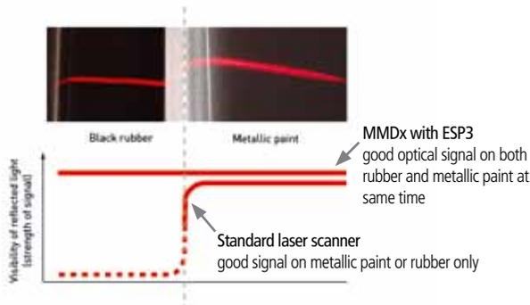
ModelMaker scanners also feature an intelligent anti-reflection filter to provide accurate measurements when scanning very shiny or polished materials. The functionality filters out all reflective laser light that is scattered in many directions.
