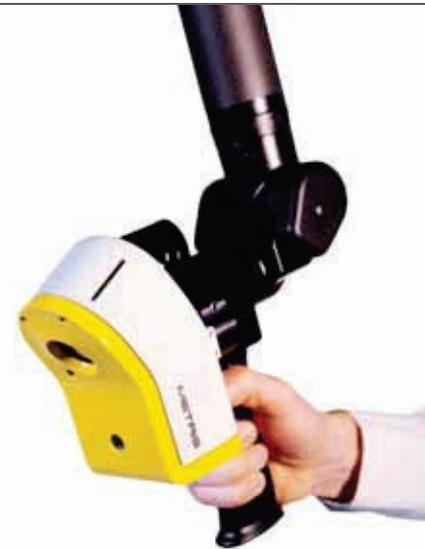
LC60Dx or LC60D CMM scanner users can extend their measurement capability by also using the scanner on an MCx arm. Refer to LC60Dx brochure for details.
