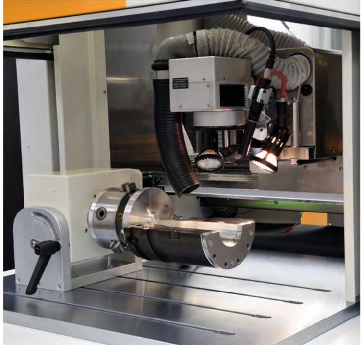
The Sisma Laser System specific for 2D and 3D deep engraving on moulds, matrix, punches and electrodes through movement of the laser source on a portal with 3 axis with a range of 350 mm. The centering is done through an high resolution ultra compact camera; working cycles, positioning and programming are managed from the master software.
