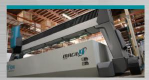
With durable design throughout, the Mach 4 is made up of precision machined and thermally stress-relieved solid steel castings, easily handling even the most rigorous use day in and day out.
