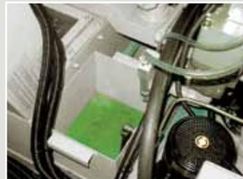
*Fluid reclamation and filtration systems separate valuable coolant for reuse - reducing waste and improving the environment.*
