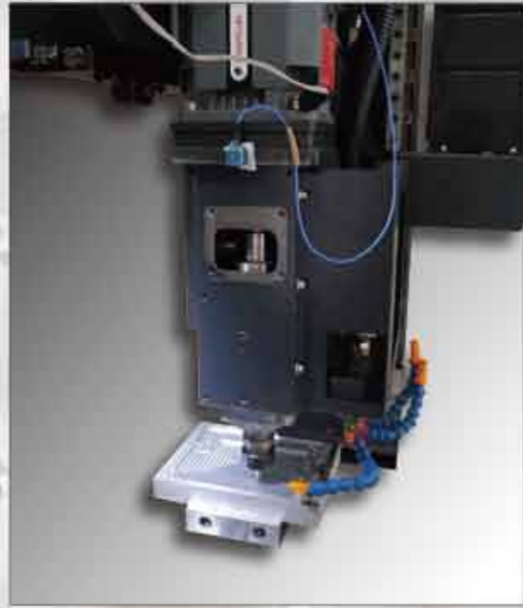
Spindle Vibration Test in Y Direction
