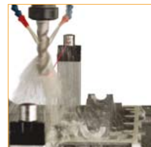
NC4 high speed non-contact laser device available as fixed or separate systems
